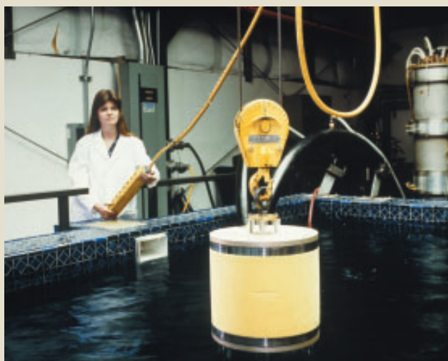
Figure 14 A technician moves a container of fruit above a pool that is used to study food irradiation. The pool contains an accelerator that produces X-rays.
