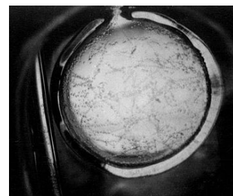
Illustration 3: A hydrogen bubble chamber image.
