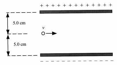
A) If the electric field is 20.0 N/C how much far will the electron travel verticaly as it passes between the plates.
