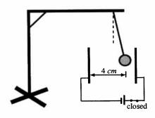
A 10 gram charged pithball is hung between the plates. When the switch is closed it moves 1.0 cm closer to one of the plates.
