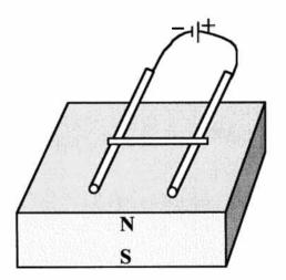
The diagram below represents an artificial heart. It works by pulsing the electric field causing the positive and negative ions in the blood to move toward the electric plates. This creates a motion of the ions perpendicular to the magnetic which creates motion along the vessel.
