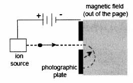
$^{12}C^{2+}$  ions are deflected in an arc of radius 0.165 m. What type of ion travelling at the same speed could be detected at a radius of 0.550 m? x indicates mass
