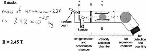
70. You are an atomic scientist and you have been given a pure sample of protactinium. Your task is to determine the ratio amounts of the isotopes using a mass spectrometer.
