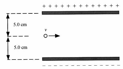
The particle has a mass of  $3.50 \times 10^{-5}$  kg and it moves horizontally to the right through the electric field of 75.0 N/C and under the influence of gravity. Using appropriate formulas and a logical method, find the net vertical force on the particle while it is travelling through the electric field.
