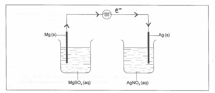
Identify the missing component of the cell and its function.
