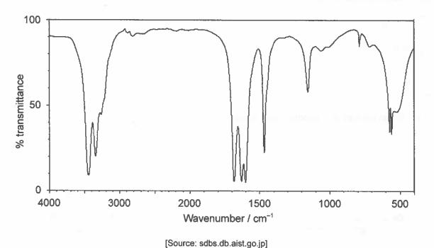
Identify the bonds causing the absorptions at 3450 cm<sup>-1</sup> and 1700 cm<sup>-1</sup> using section 26 of the data booklet.
