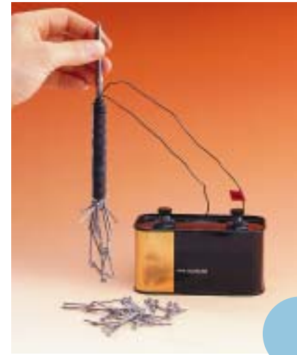
Figure 3.9 An electromagnet is made by winding a current-carrying wire around a metal core.
