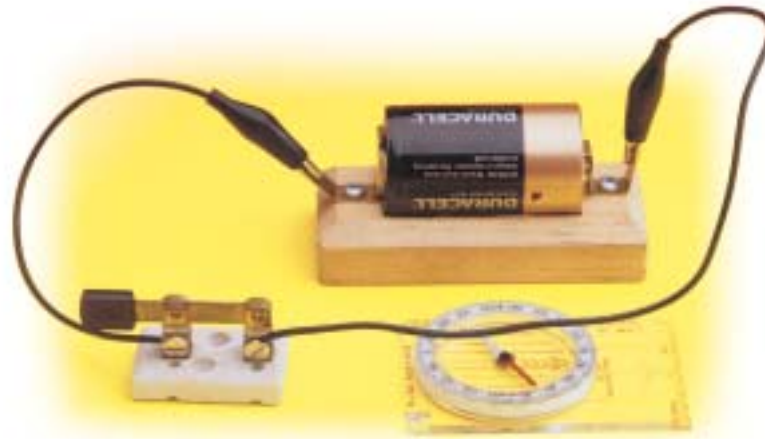
Figure 3.7 Electricity flowing through the wire causes the compass needle to deflect.
