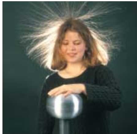
Figure 1.4 A Van de Graaff generator uses friction to build up a static charge on its sphere.
